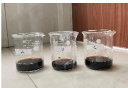
Fig 2. Results of the Synthesis of C-Dots A, C-Dots B, and C-Dots C Using the Agitation Method
